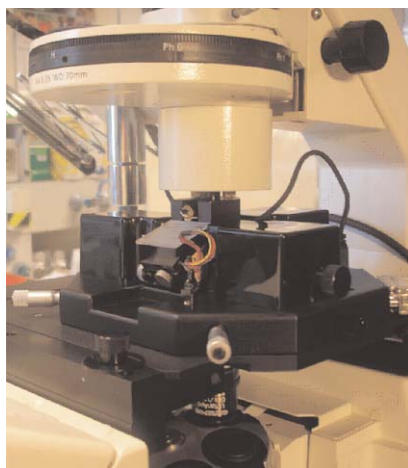
Figure 2. Agilent 5500 ILM AFM/SPM with a Zeiss Axiovert 200 inverted light microscope. The 5500 ILM AFM/SPM is also compatible with other inverted light microscope makes and models.
